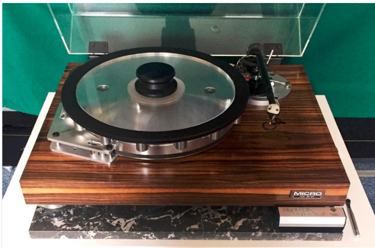
Fig. 1: The Micro Seiki BL 91 record player with centre Puck en platter "ausen" stabilizer ring
