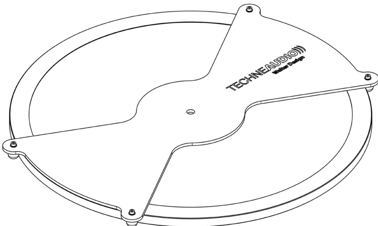
**Outer ring with centering propeller
